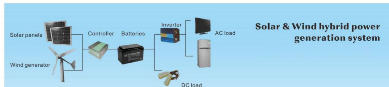
Configuration diagram of Solar and wind power generation system
